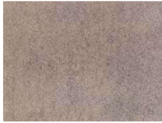
Condition B Blasted to Sa2.5
