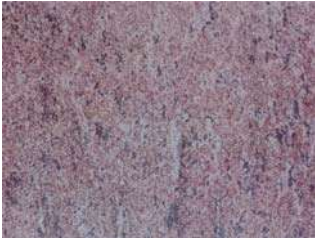
Condition A Blasted to Sa1
