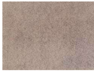
Condition C Blasted to Sa2.5
