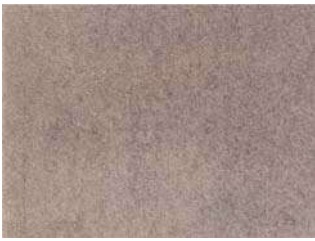
Condition A Blasted to Sa2.5
