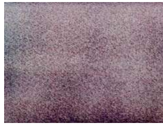
Condition C Blasted to Sa2
