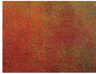
Condition C Blasted to Sa1
