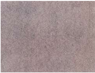
Condition A Blasted to Sa2
