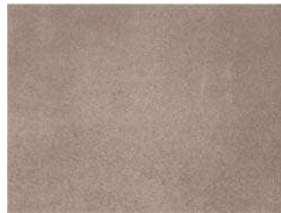
Condition C Blasted to Sa3
