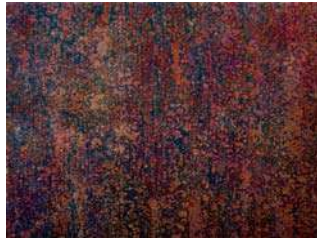
Condition B Blasted to Sa1
