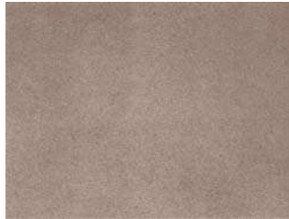
Condition B Blasted to Sa3
