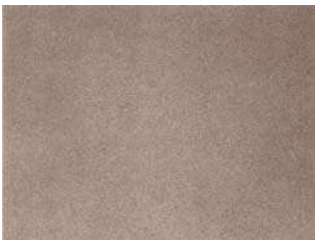
Condition A Blasted to Sa3
