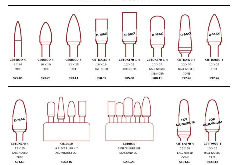
**DIAMOND CUT** is a universal cutting style offering smooth operation with a high cutting action. **D-MAX** have an extra strong tooth formation making them ideal for fast, heavy duty stock removal. **ALUMINIUM CUT** provides rapid stock removal on softer materials like Aluminium, Brass, Plastics etc.
